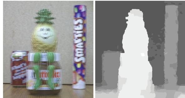
**Fig. 1.** Left: Image captured using a coded aperture camera. Right: Depth map recovered by our algorithm given the single image at the left as input (white indicates closer objects).
